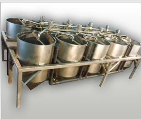
Tank Farms, Corn Soak Systems
