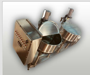
Mixing Use Tank Skid
