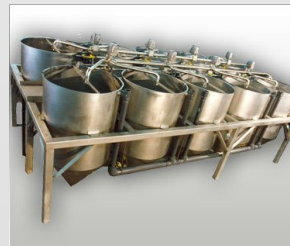
Tank Farms, Corn Soak Systems
