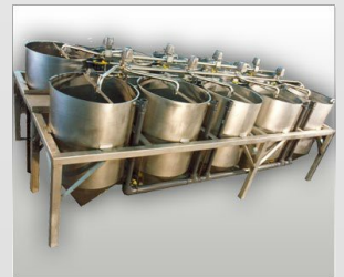
Tank Farms, Corn Soak Systems
