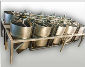
Tank Farms, Corn Soak Systems
