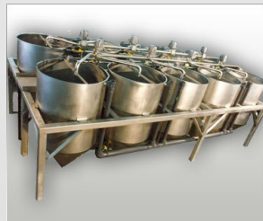
Tank Farms, Corn Soak Systems
