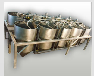
Tank Farms, Corn Soak Systems
