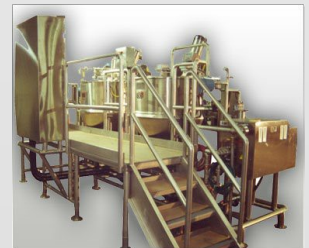
Mix Use Tank Slurry Systems
