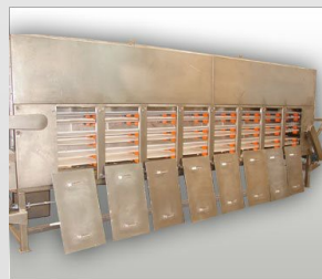
Multi Tier Cooling Conveyors
