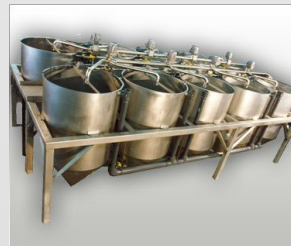
Tank Farms, Corn Soak Systems
