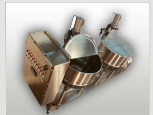
Mixing Use Tank Skid
