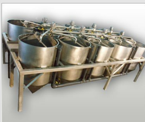
Tank Farms, Corn Soak Systems
