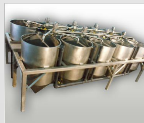
Tank Farms, Corn Soak Systems
