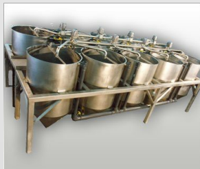
Tank Farms, Corn Soak Systems
