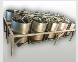
Tank Farms, Corn Soak Systems
