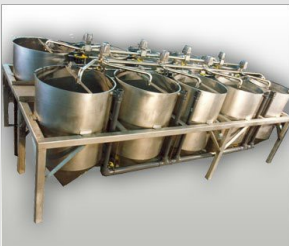
Tank Farms, Corn Soak Systems
